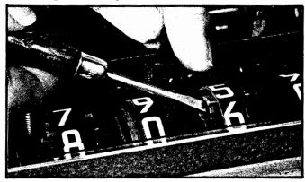
Figure 6-8 Removing Insert from Notch on Second Wheel.
